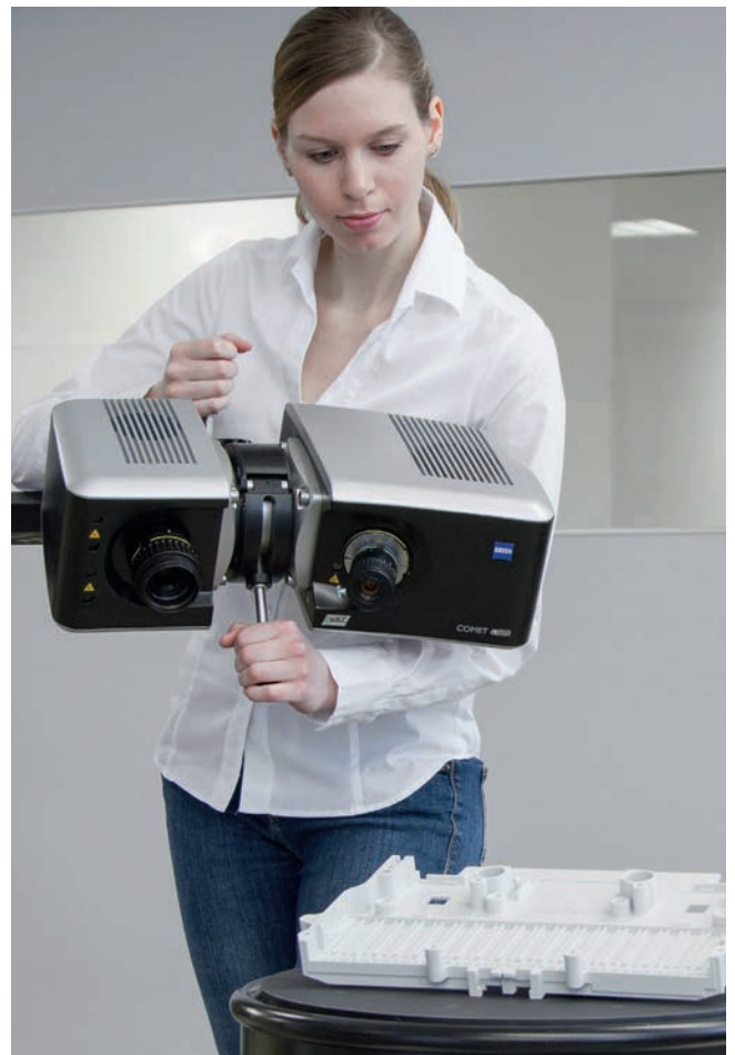
The user-friendly handling unit enables the ZEISS COMET 6 sensor to be positioned especially easily and quickly.
