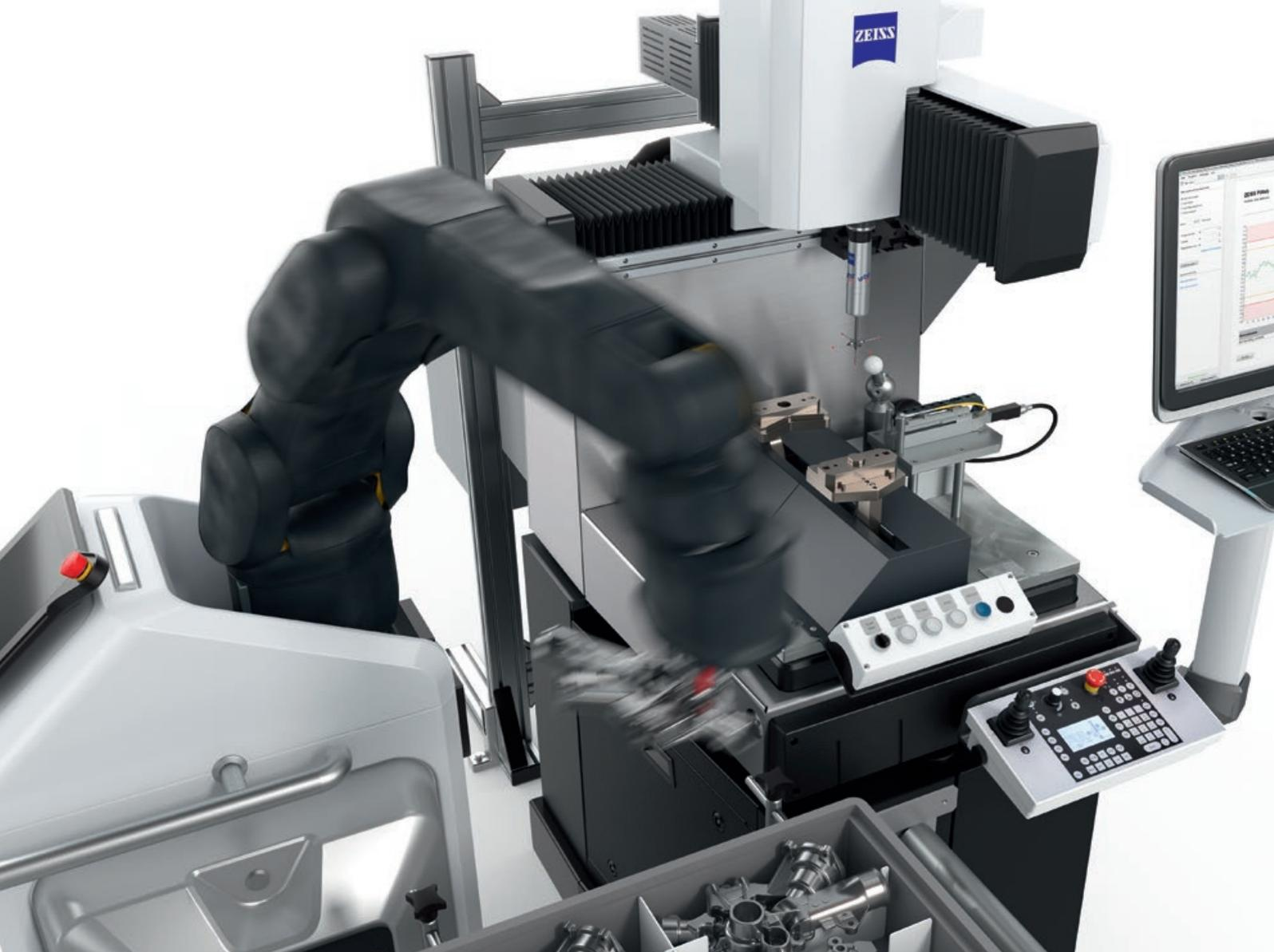
*The flexible measurement system, consisting of a collaborative robot and a ZEISS DuraMax HTG, reduces the metrology engineer's day-to-day workload while simultaneously increasing productivity.*
